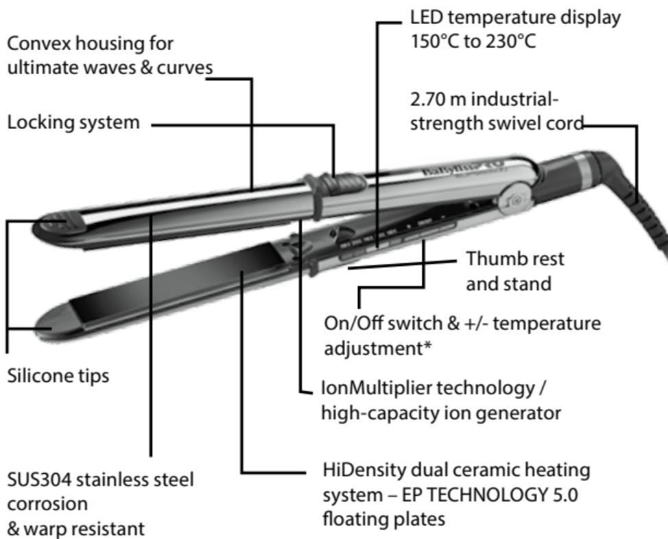
\* Press and release to turn on – Press and hold for a second to turn off
